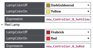
7 Drag-and-drop a Momentary Button Object from Toolbox into the Page as the button is overlaid on the Bit Lamp Object.
